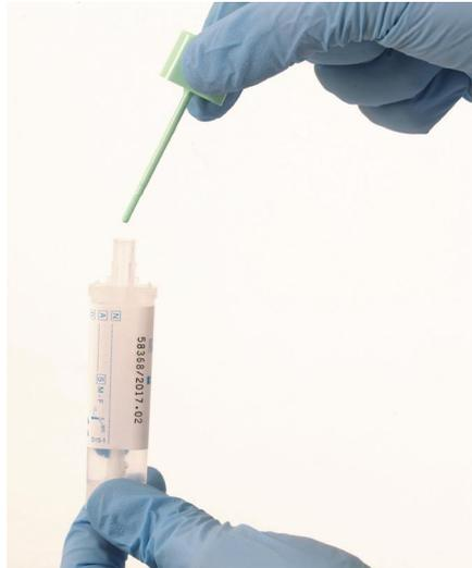
Unique sample collection device, complete with an integrated sample filter.
